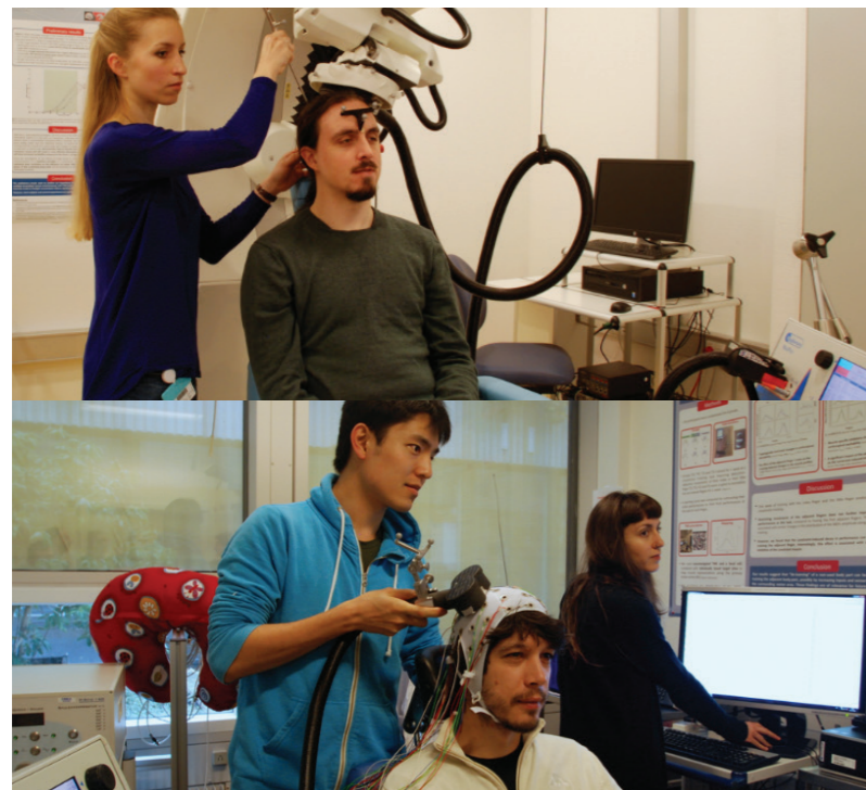
Top image: Registering a participant in the newly acquired TMS-robot that allows for precision targeting and mapping. // Bottom image: TMS-EEG experiment
